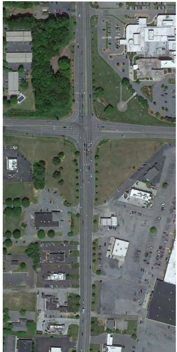
The intersection improvement that is planned for Kings Highway and Van Buren Road (TIP Project Number U-5893) will improve traffic flow along two main arterials in the City of Eden. The project may leave unused right-of-way in all four quadrants as it was originally envisioned to be an interchange. This right-of-way is an opportunity for beautification or infill development.
